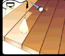
Apply IN-WOOD with a brush, roller, or sprayer working lengthwise. Stain only as many deck boards at a time as you can comfortably reach to maintain consistency
